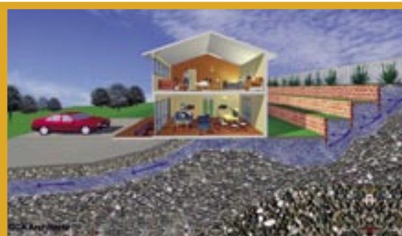
Typical slab on ground construction requires earthworks to establish a level site for the house. Retaining walls may affect natural groundwater flow. Terraced areas may be made of saline soils. The house slab prevents evaporation from the soil surface while increasing the opportunity for salty water to enter the structure.
