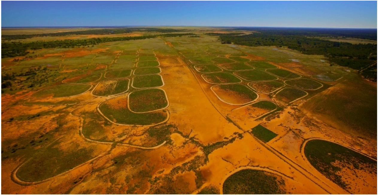
Figure 5 Scald reclamation area showing water ponding trials
