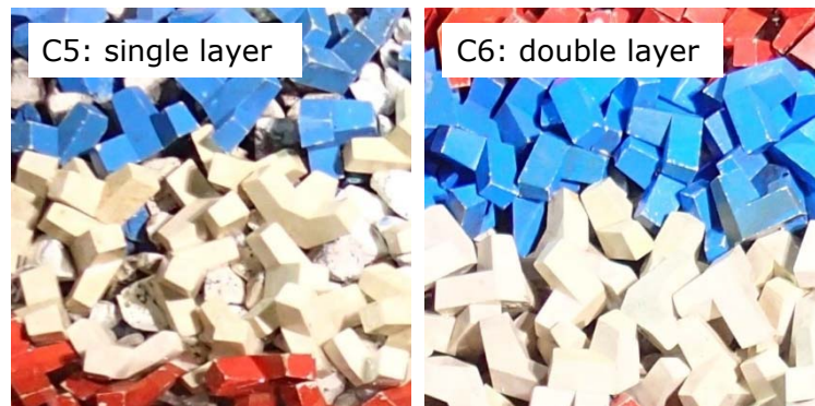
Figure A.9. Comparison of single and double layer Hanbar armour
