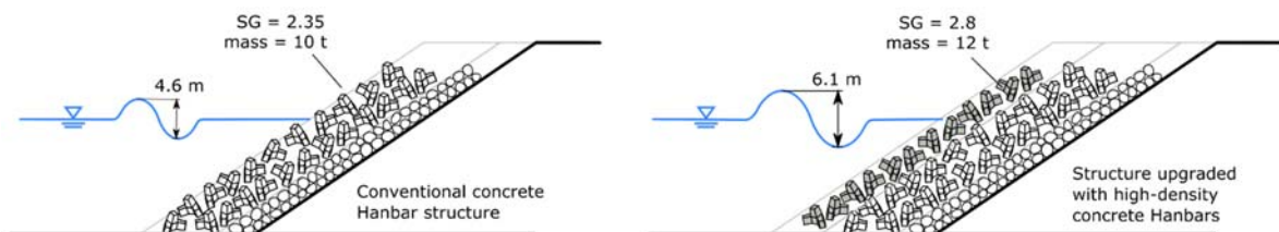
Figure 7.4. Upgrading an existing structure with one layer of high-density concrete Hanbars
