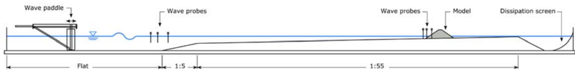
Figure A.1. WRL 3 m wide wave flume
