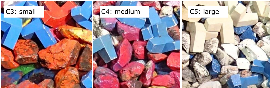
Figure A.8. Underlayer rock ratios for single layer Hanbar models (after failure)
