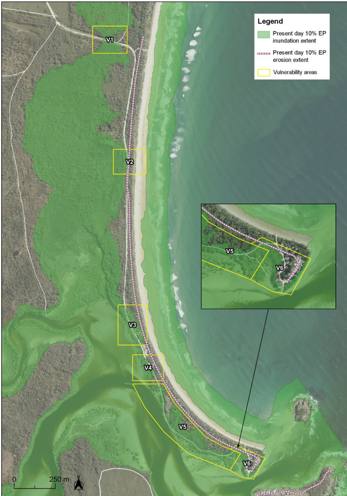
Figure 8 Coastal hazard vulnerability zones V1 to V5 (along Sandon River Road) and V6 (Sandon River campground area) for present day (2024) inundation and erosion events
