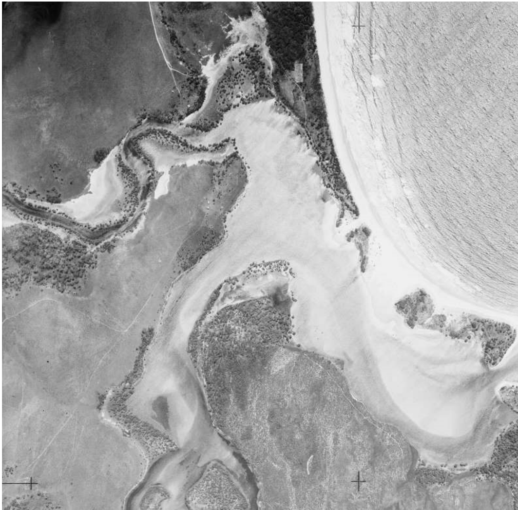
Figure B.1 1942 – showing potential wave overwash at 2 locations and substantial sand accretion along Sandon Beach and within Sandon River
