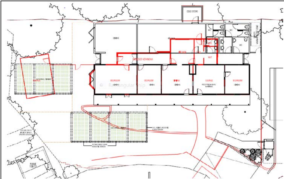
Figure 60 – Demolition plan Source: Johnson Pilton Walker
