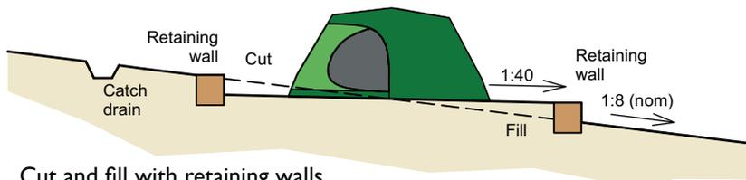
Cut and fill with retaining walls
