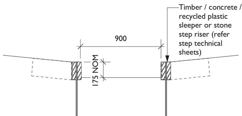
**Cross section – walk-through drain**
