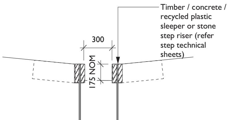
**Cross section – step-over drain**
