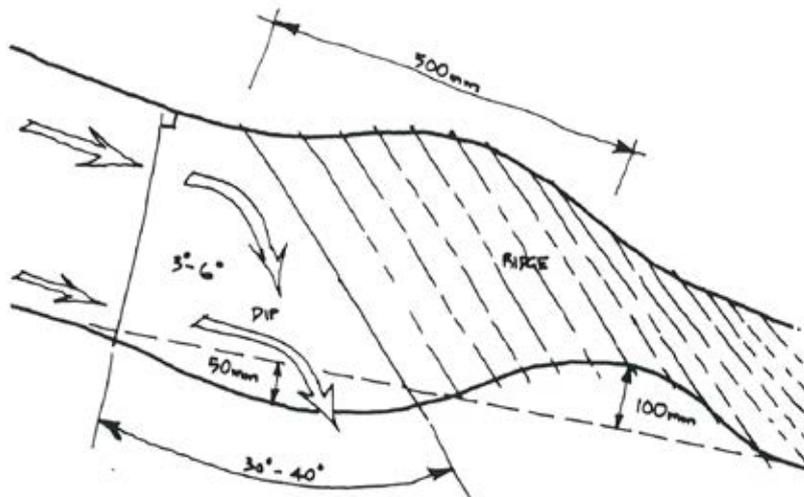
Use hard stable soil – cement stabilised clay/gravel if necessary
