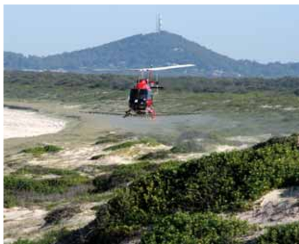
Aerial boom spraying along a beach from a 12 m wide boom
