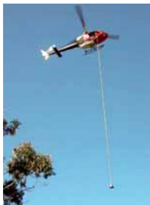
Spot spraying using a conical device suspended from a helicopter
