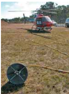
Spot spraying using a conical device suspended from a helicopter
