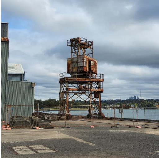
Figure 214: Cruiser Wharf Travelling Jib Crane, Crane Number C60, with jib removed since 2019 for safety. Source NPWS/Ed Beebe Nov 23
