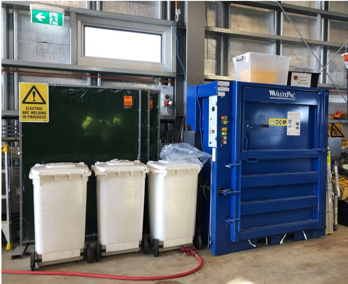
Image 5 Soft plastic baler in the NPWS Perisher Valley Waste Transfer Station. Photo: E Stafford/DCCEEW
