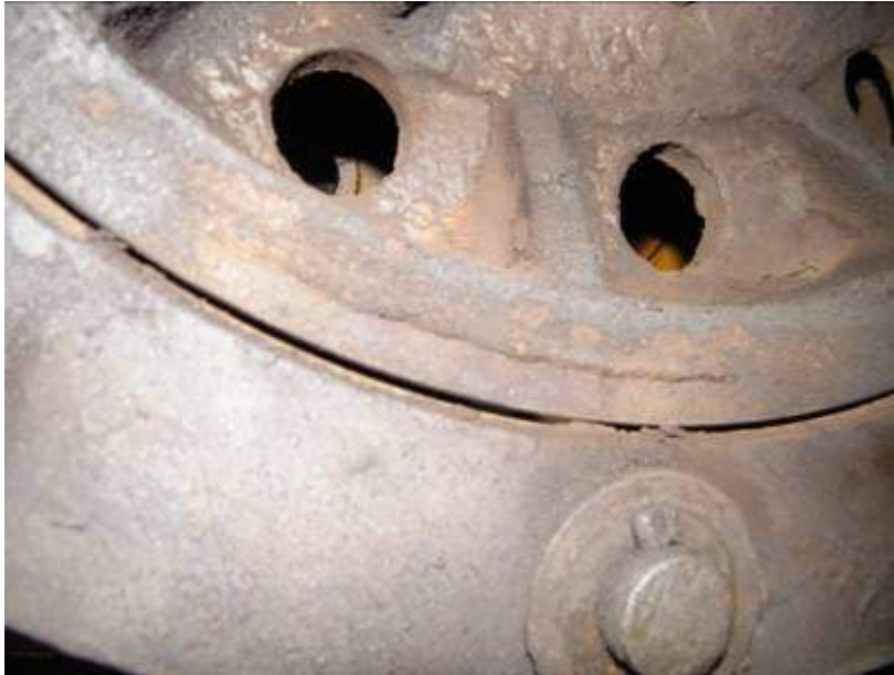
Figure 11 Main Winch Brake - Brake pad material requires replacement
