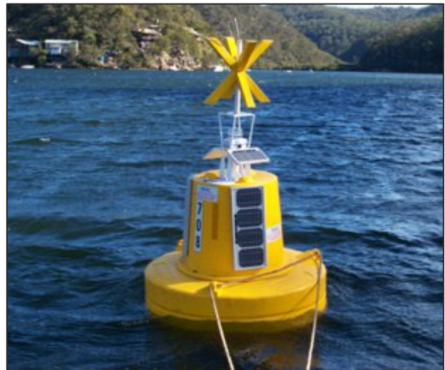
Image: water quality buoy (source: https://mhl.nsw.gov.au/DataCollection )
