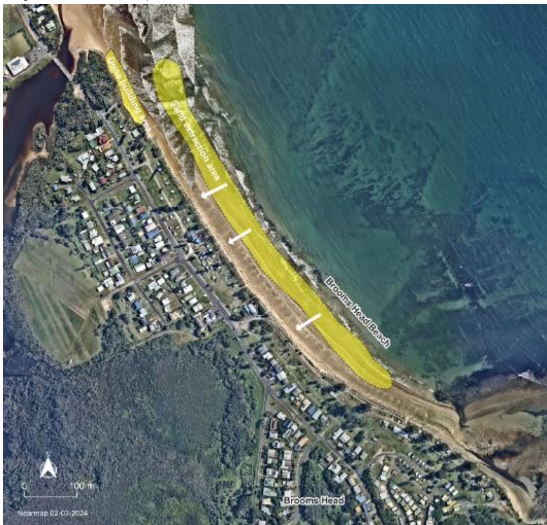
Figure 51: Indicative beach scraping at Brooms Head to be accompanied by dune fencing and rehabilitation
