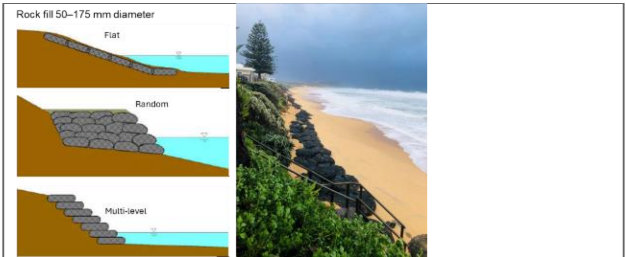
Figure 54: Rock bag revetment wall, left: typical rock bag deployment methods (Bluemont), right: rock bags at Wamberal Beach (image: Bluemont)
