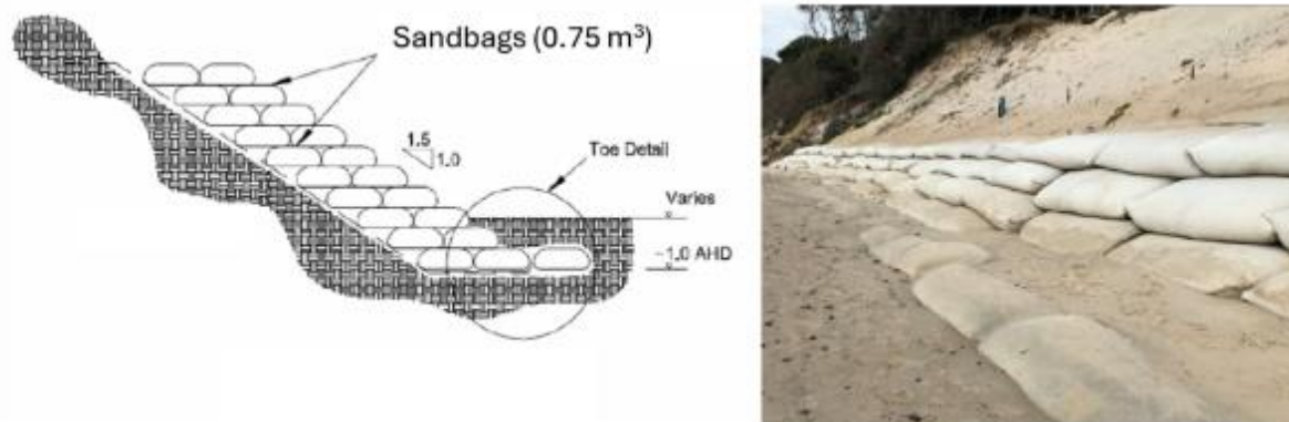
Figure 53: Sandbag revetment wall – left: typical cross-section (revetment height varies, adapted from Coghlan et al. (2009)), right: sandbag revetment wall at Clarkes Beach, Byron Bay (image: J. Carley)
