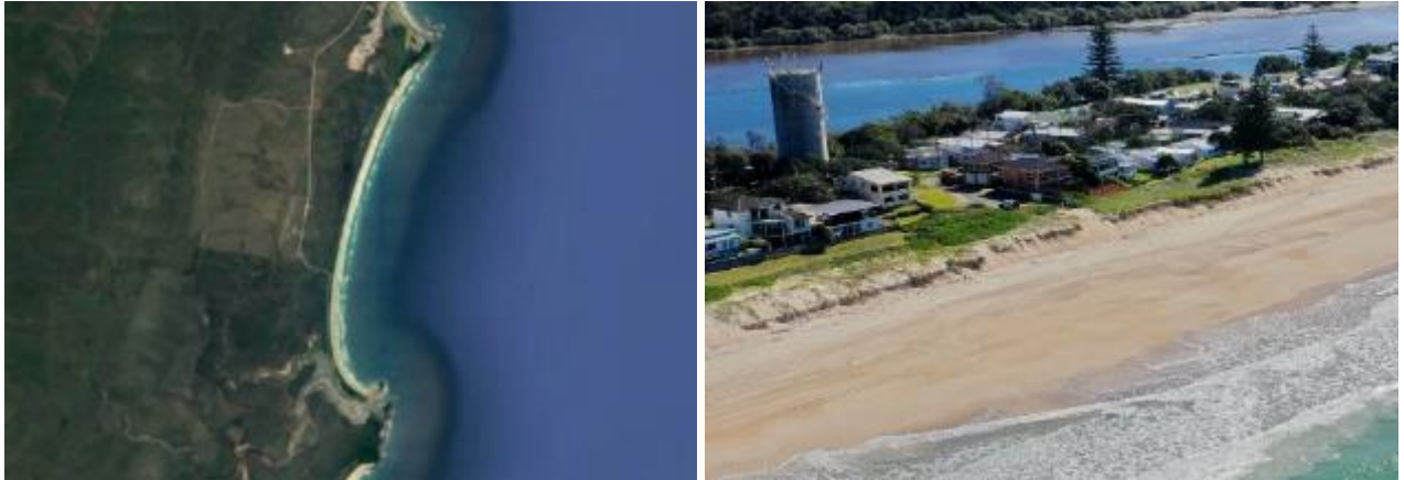
Plate 3: Example coastal processes: Left: crenulate shaped beach at Sandon, right: erosion at Wooli
