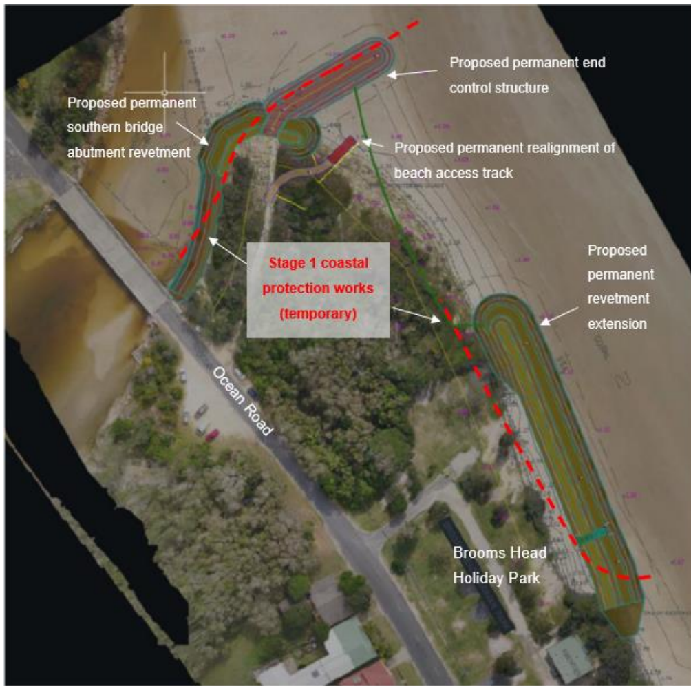
Figure 52: Potential locations for stage 1 coastal protection works (temporary) to be confirmed through design and approvals – Brooms Head
