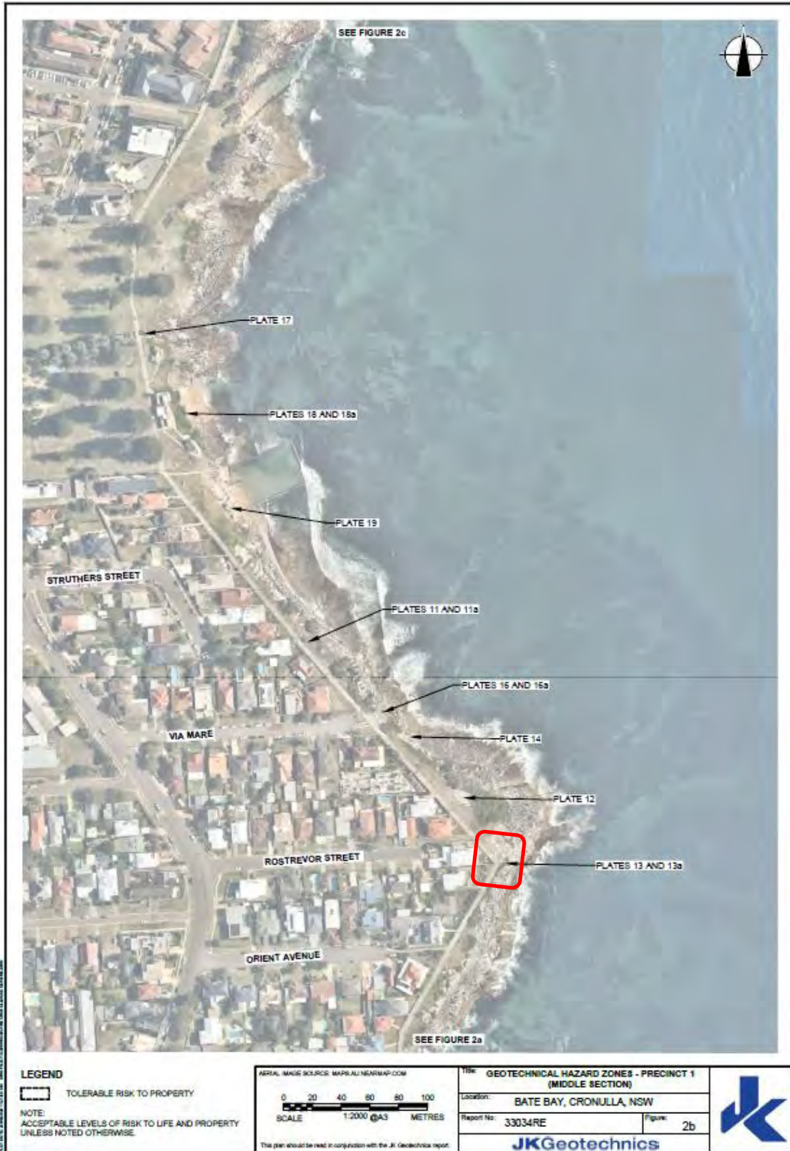
Figure 17-9: Geotechnical Hazard Zones - Precinct 1 (Middle Section) (key location marked in red)
