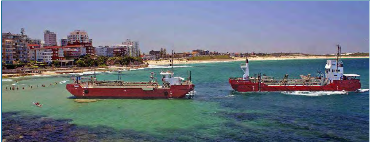
Figure 8-6: Port Frederick and Faucon hopper dredges placing sand at Cronulla Beach (from Port Hacking dredging) through split hopper bottom dumping, circa 2003
