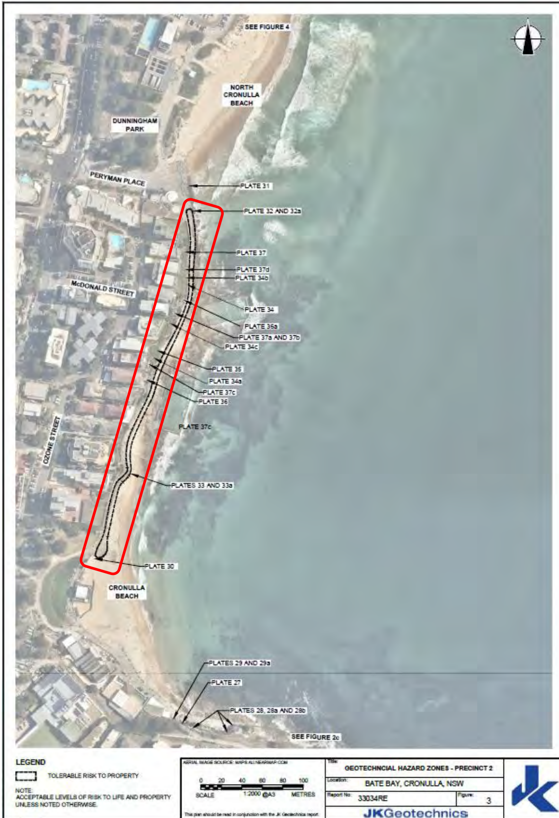
Figure 17-11: Geotechnical Hazard Zones - Precinct 2
