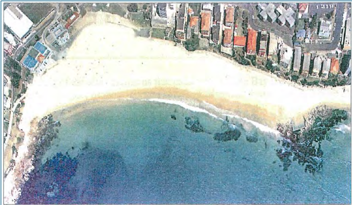
Figure 8-5: The highly nourished state of Cronulla Beach at the end of August 1977, midway through the first stage of nourishment (note that the saturated subaerial portion of the beach filled in adjacent rockpools) (Patterson Britton, 2006)
