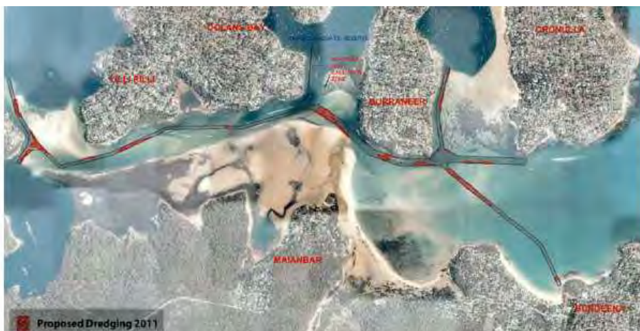
Figure 8-10: Proposed 2022 dredging configuration to maintain viability of navigation channels (source: Council, 2021)
