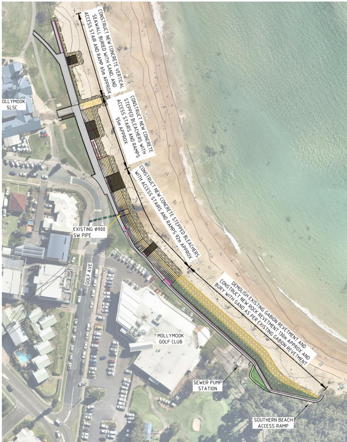
Figure 4-33 Concept Design of South Mollymook Coastal Protection Works (Advisian, 2022)
