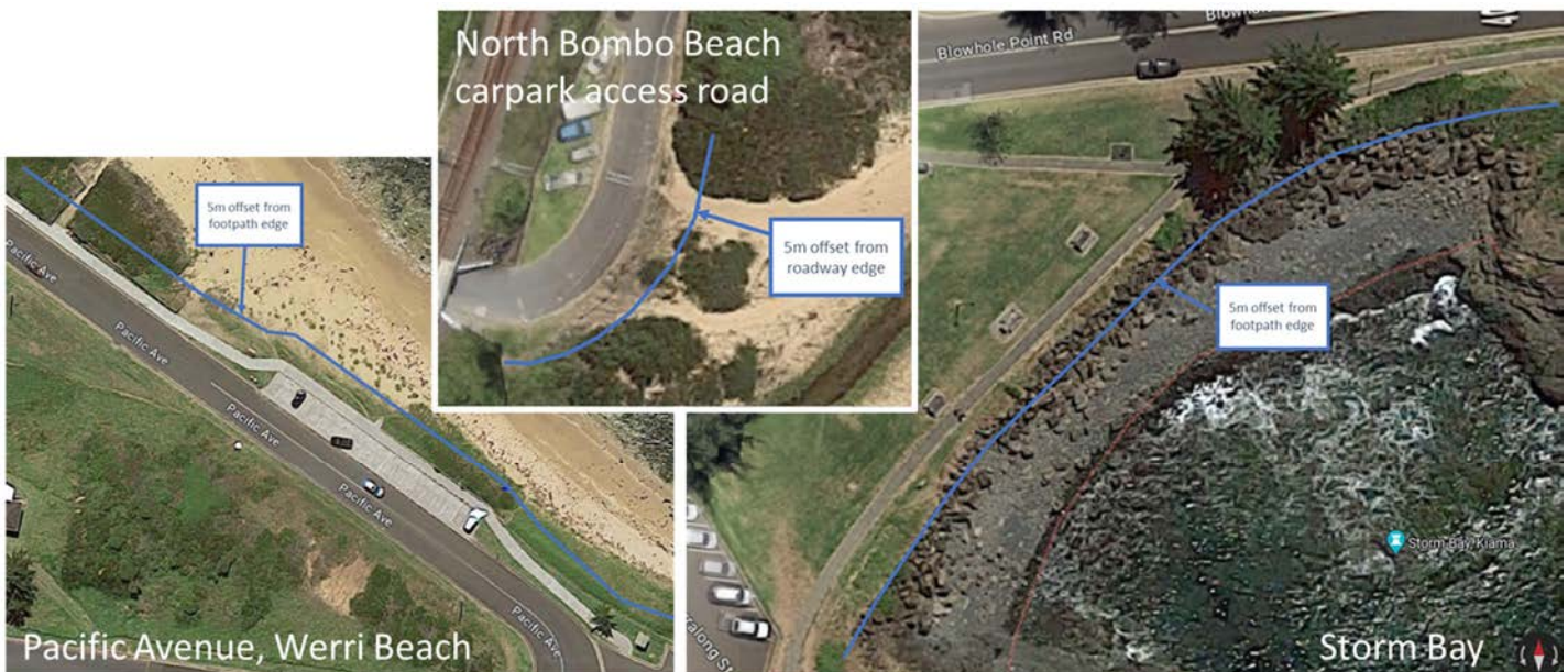
Figure E.1 Approximate locations of erosion scarp to reach trigger and threshold (to be confirmed through REF and approvals process) (Source: Google)
