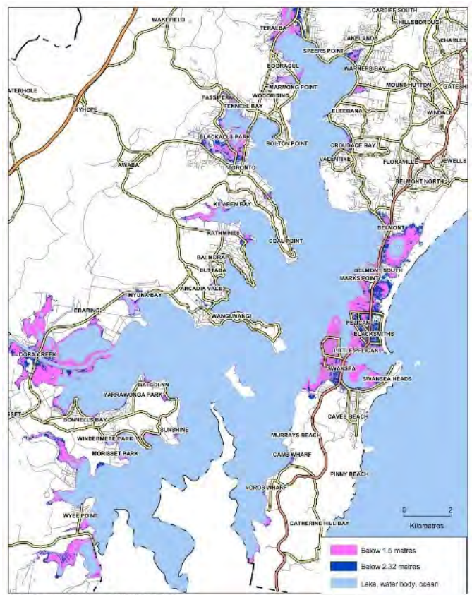
Figure 11: Low-lying areas affected by inundation
