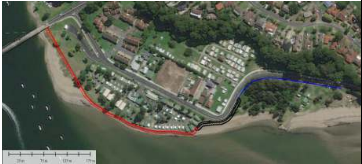
Figure 2 Alignment and extent of Stage 2 Inundation Protection of Wharf Road (Red: Raising of Seawall, Blue: Vertical SSP).
