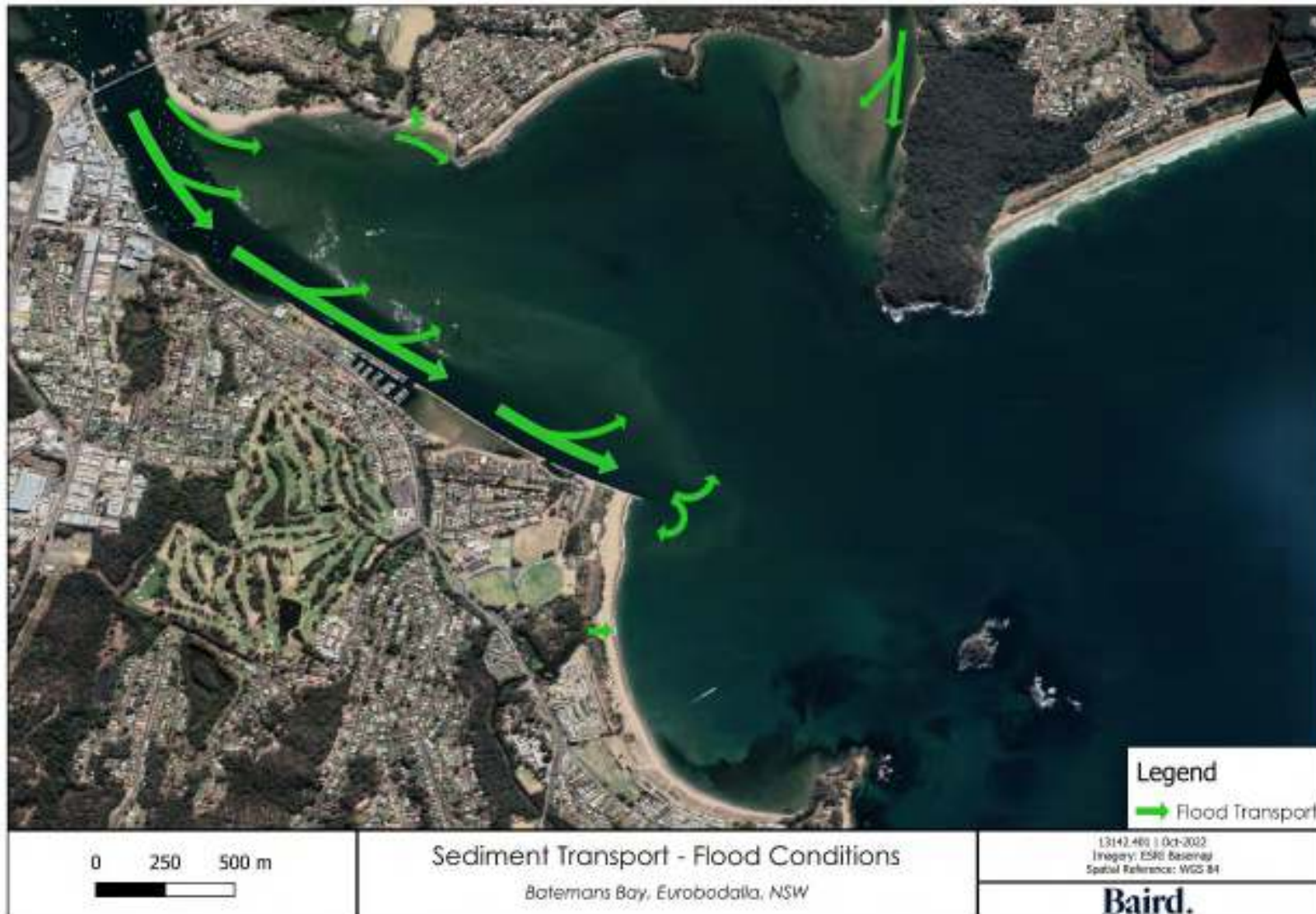
Figure 6-9 Conceptual sediment transport model of inner Batemans Bay under catchment flood conditions
