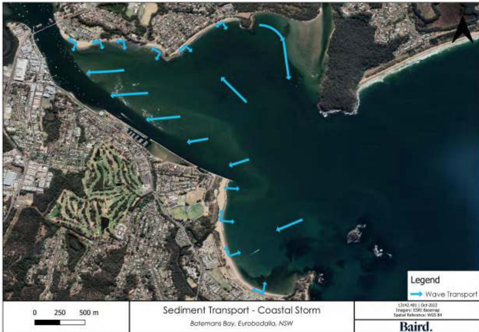
Figure 6-8 Conceptual sediment transport model of inner Batemans Bay under coastal storm conditions
