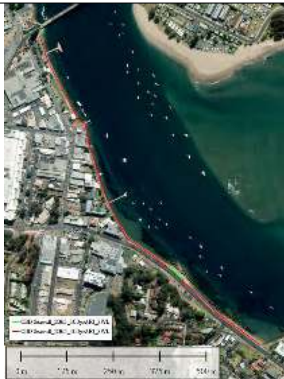
Figure 2 CBD Seawall Inundation for the 100year ARI still water level at 2065 (red = existing seawall crest submerged)
