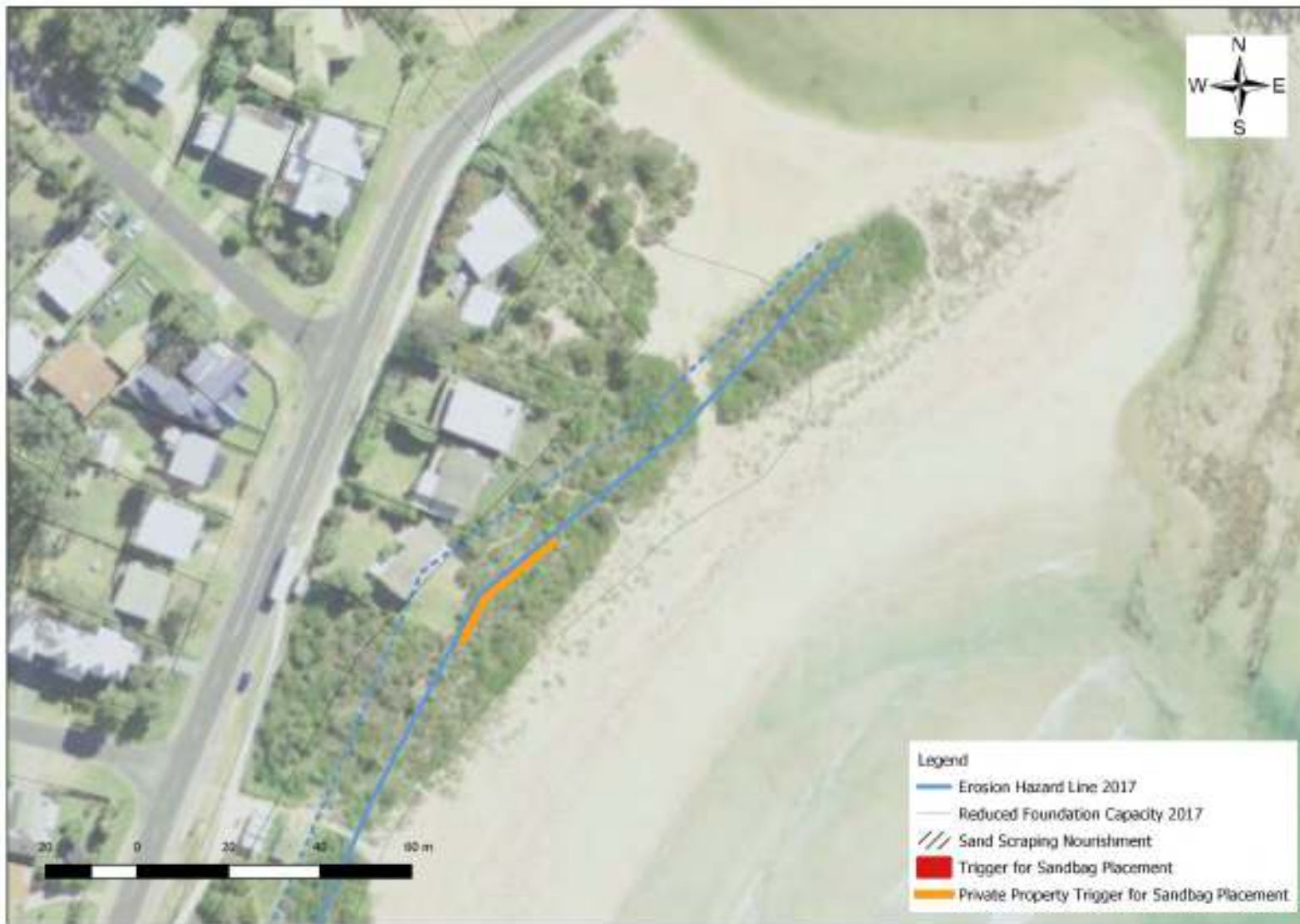
Figure 5-9 Broulee Erosion Protection Works
