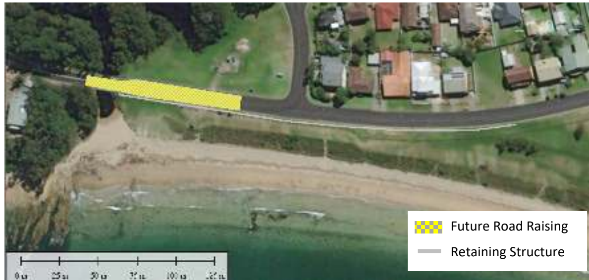
Figure 3 Alignment and extent of Road Raising and retaining structure at Maloneys Beach
