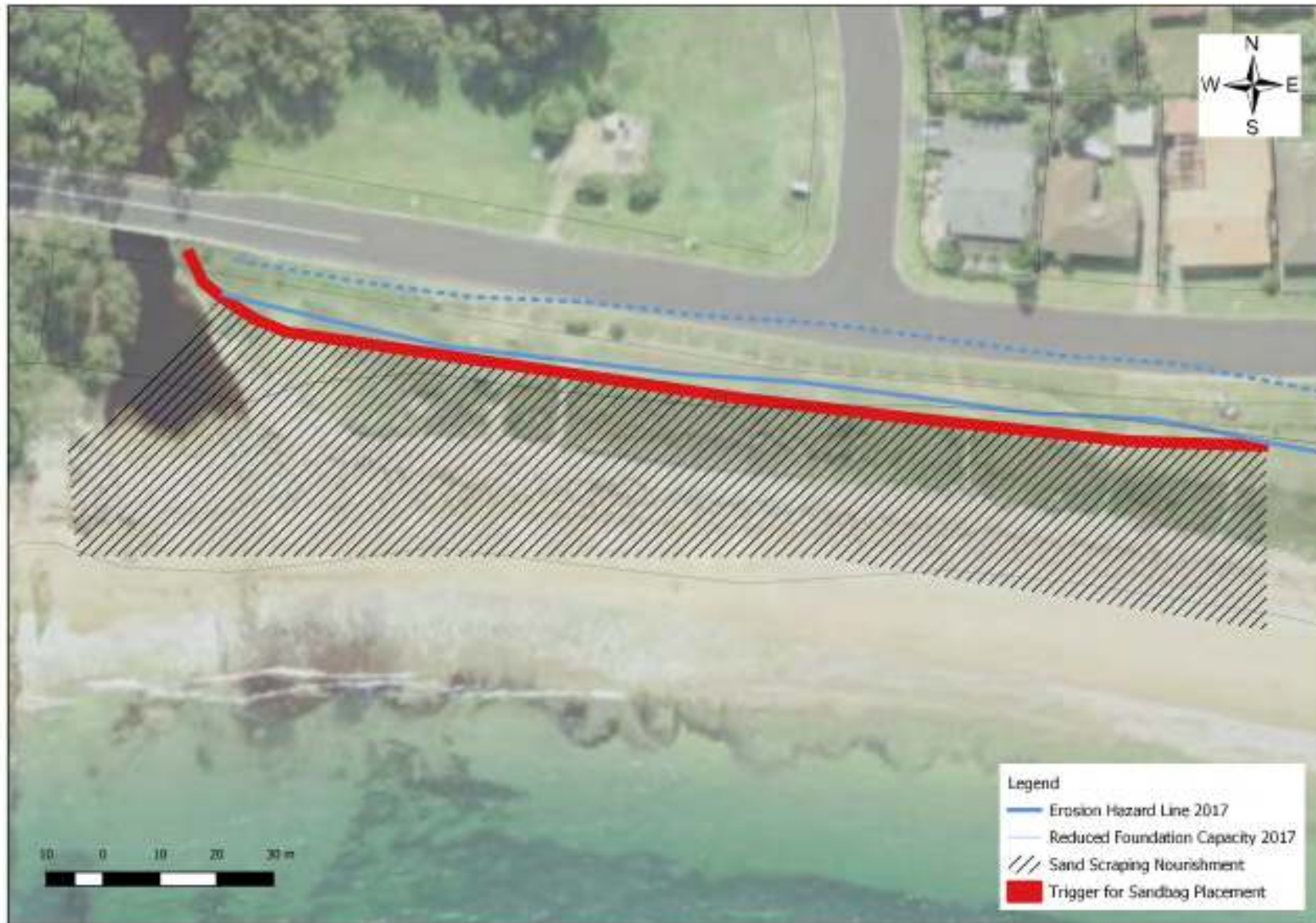
Figure 5-2 Malneys Beach Erosion Protection Works
