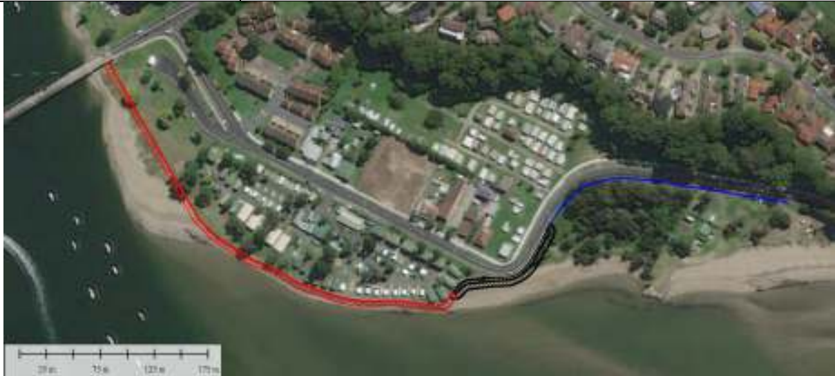
Alignment and extent of Stage 2 Inundation Protection of Wharf Road (Red: Raising of Seawall, Blue: Vertical SSP)
