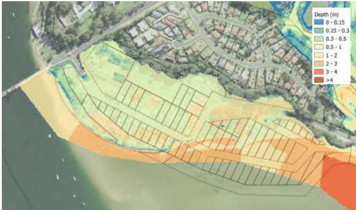
Figure 1. 100year ARI Coastal Inundation Depth across Wharf Road area. Top: Present Day. Bottom: 2100.
