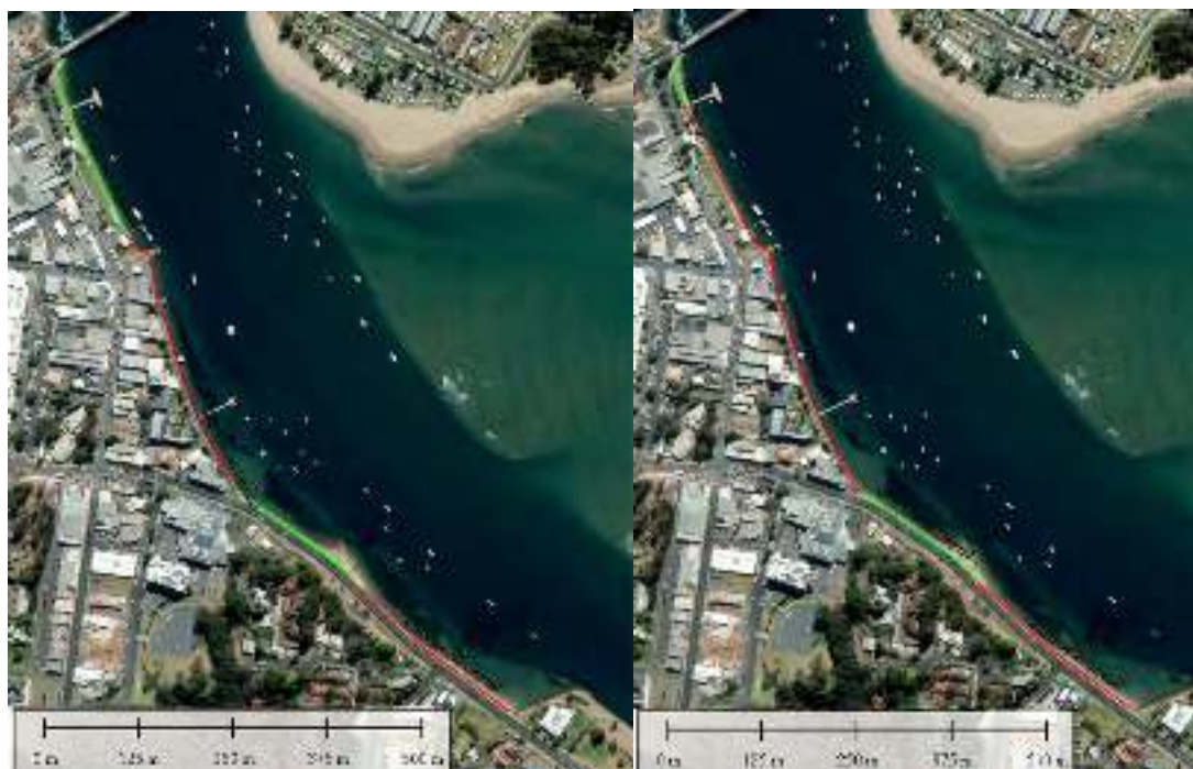
Figure 1 CBD Seawall Inundation for the 100year ARI still water level under present day sea levels. Left: 20year ARI. Right: 100year ARI (red = existing seawall crest submerged)
