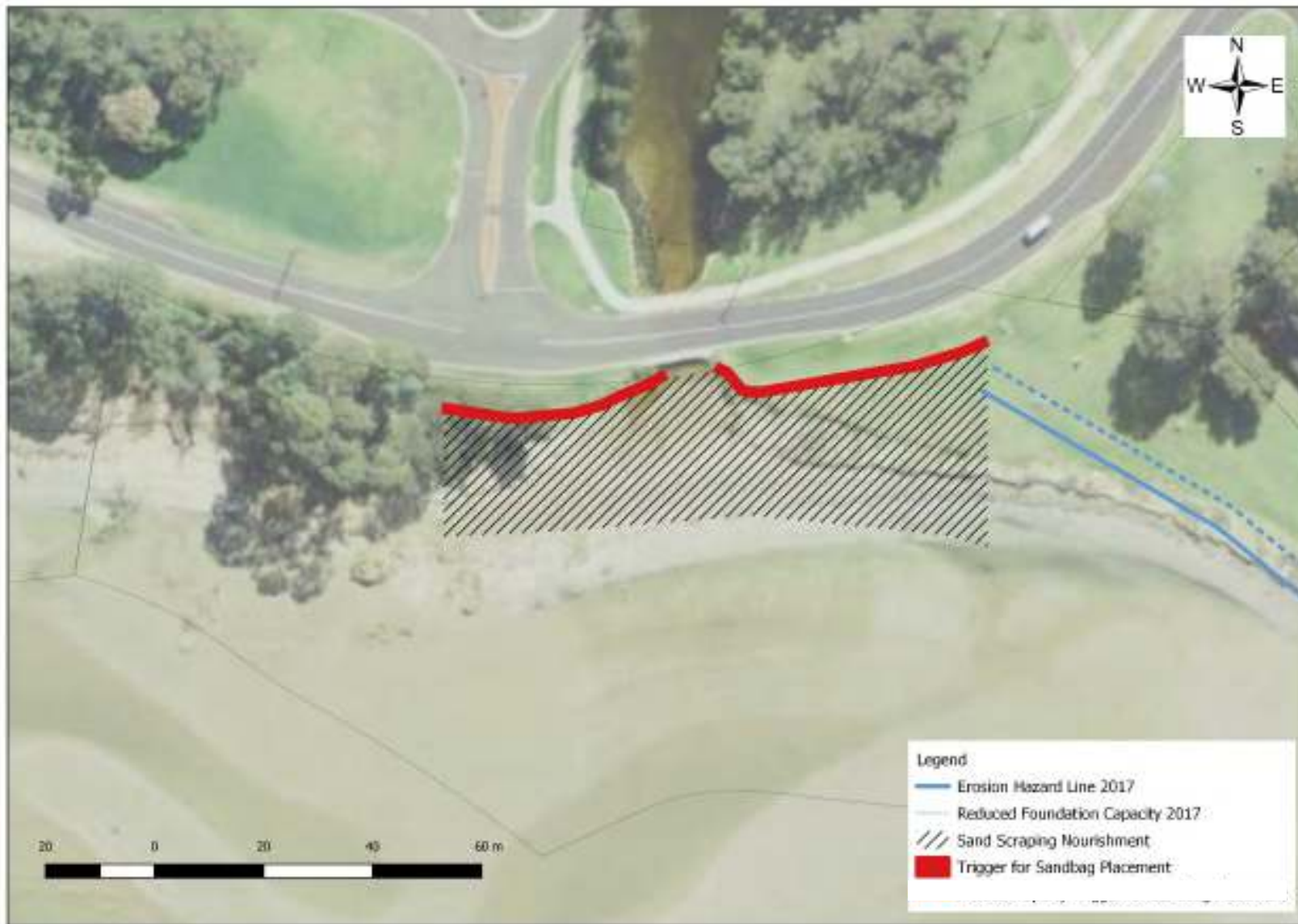
Figure 5-4 Surfside Beach Erosion Protection Works
