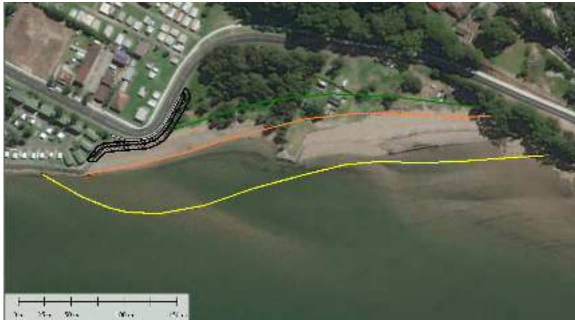
Figure 7. Shoreline positions following removal of the unapproved coastal protection structure. Green is permanent vegetation line. Orange is the receded shoreline alignment. Yellow is the accreted shoreline position.
