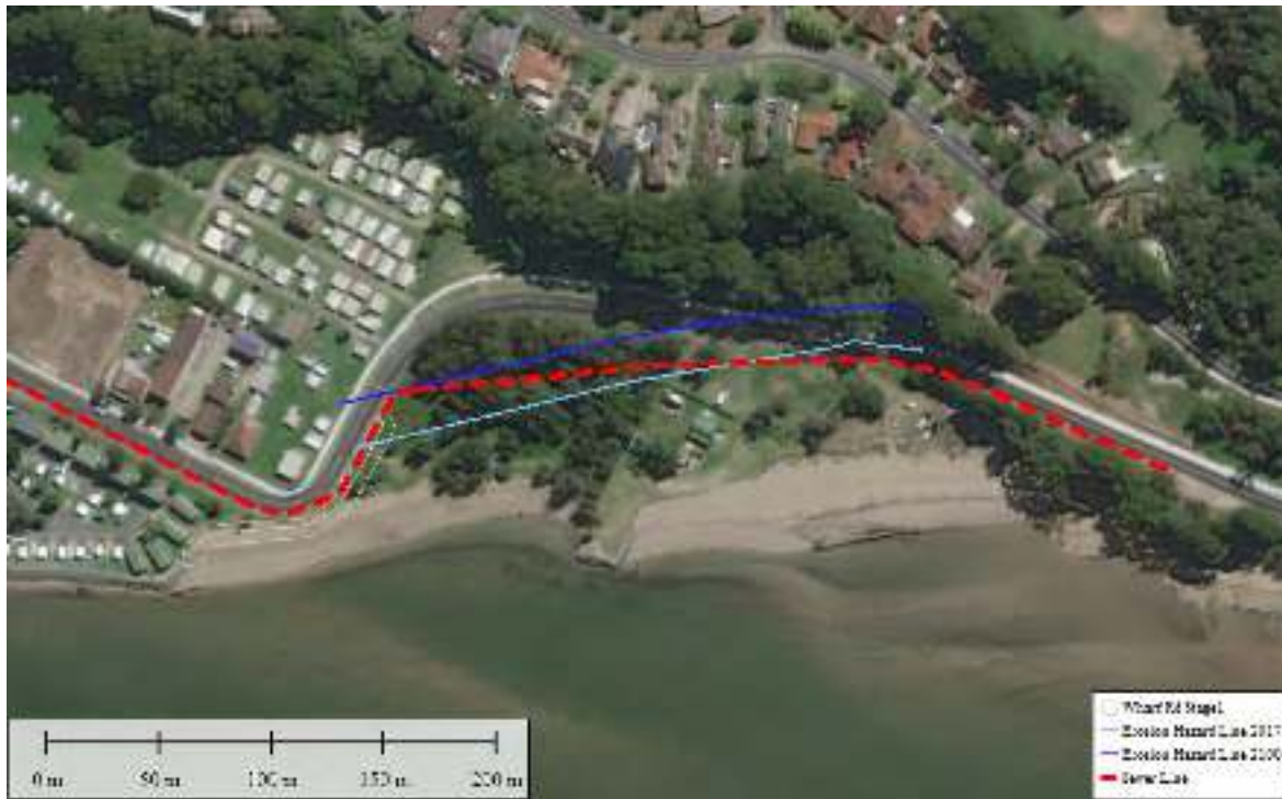
Figure 5-6 Sewer Infrastructure at Wharf Road
