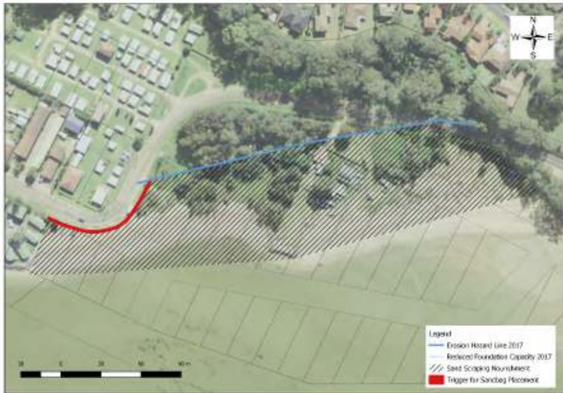
Figure 5-5 Wharf Road Erosion Protection Works
