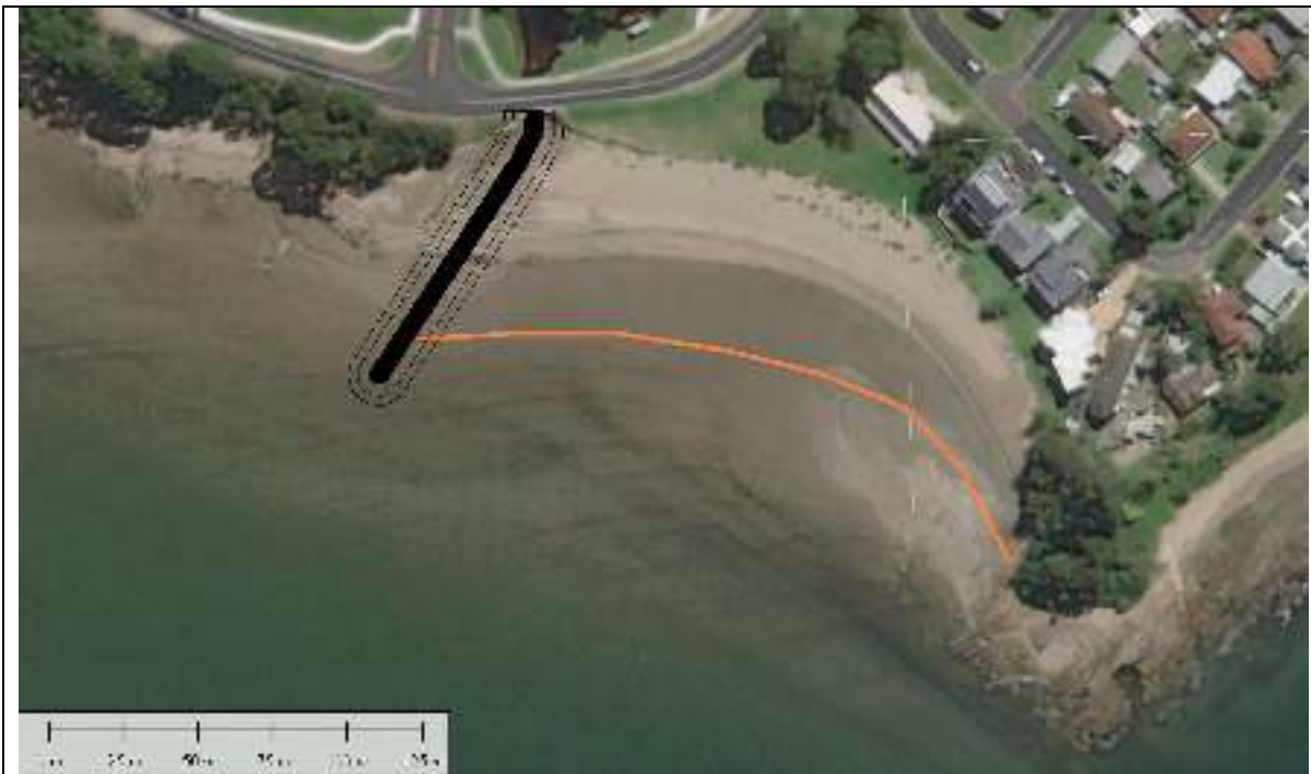
Figure 1. Indicative alignment of a culvert extension/groyne structure (black) at Macleod's beach with anticipated shoreline response (orange)
