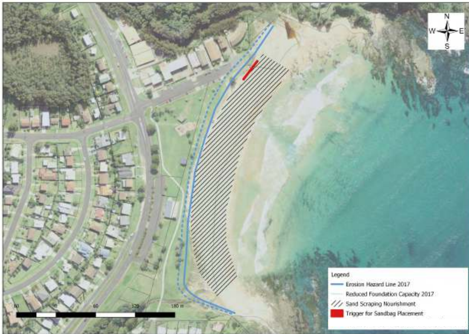
Figure 5-8 Malua Bay Erosion Protection Works
