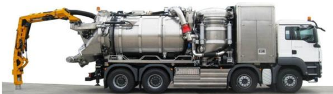
Vacuum Loader - Cap Bora Excavation Unit
